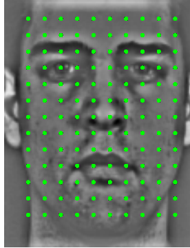
Fig. 1. Rectangular grid over the preprocessed (geometrically and photometrically normalized) face image. At each node, a Gabor jet with 40 coefficients is computed and stored.
